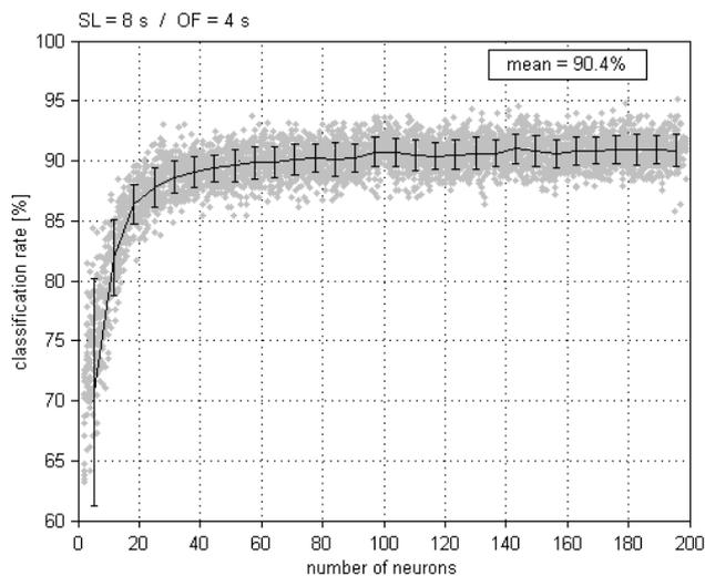
**Figure 4:** Classification rates versus number of neurons. 5,000 LVQ networks were trained and tested with different training set / test set partitions and different initializations. Mean classification rate was computed between 30 and 200 neurons.
